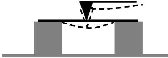
Figure 2.11 Schematic drawing of three-point bending tests using AFM.
